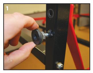
. Remove the four outside Levelers located on the bottom of the Frame Legs. See image 1.
