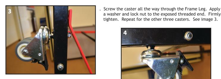
. To lock the caster into a fixed position, press down on the plastic tab. To release, pull up. See image 4.
