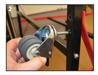
. Align and screw the caster into the threaded nut on the outside bottom of the Frame Leg. Repeat for the other three casters. See image 2.
