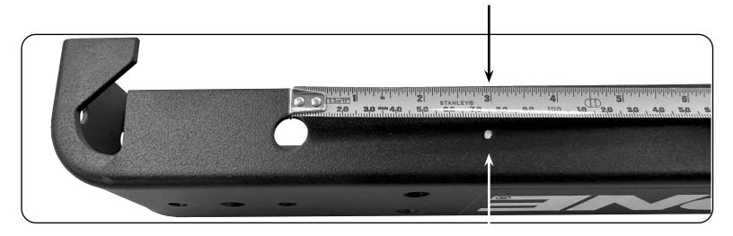
Align the mounting holes of the stabilizer to the newly drilled and pre-drilled holes in the trailer.
