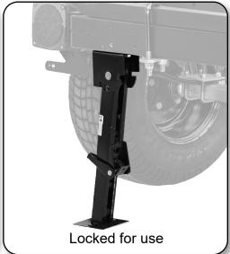
Press the brake lever to lower the telescoping section.
