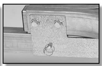
13. Add the tongue safety bolt to the bottom hole of the tongue at the non-coupler end as pictured. Tighten fully.
