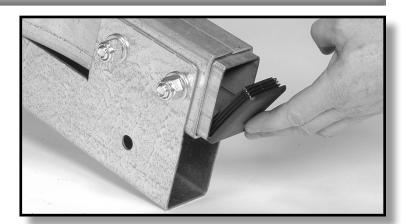
12. Tuck the rear end of the wiring harness into the end of the tongue and slide the rear end of the tongue into the retractable receiver box until the pin in the box aligns with one of the 2 pin holes in the side of the tongue. Pass the hitch pin through and install the ring clip.
