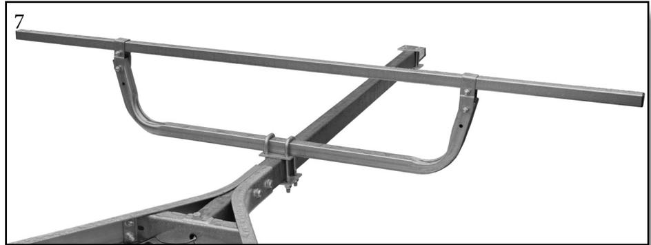
**Step 7.** Center the cross rail and fully tighten all the bolts. See Figure 7.
