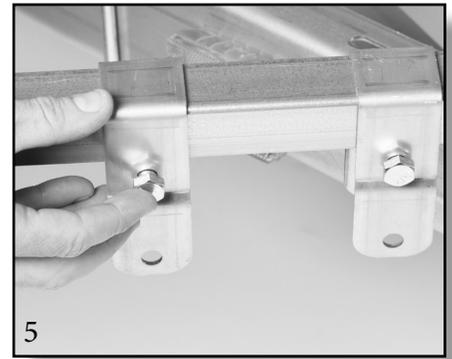
**Step 6.** Install and hand tighten the bolts holding each bracket to the support tube. See Figure 6
