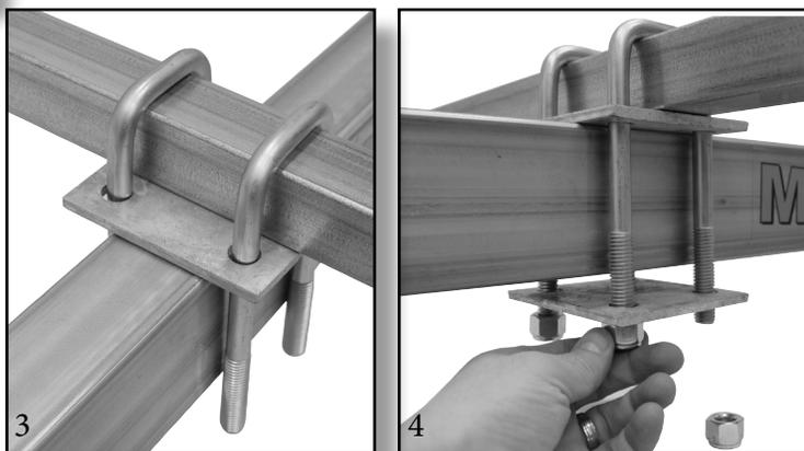
**Step 4.** Rotate the lower mounting plate and align the holes with the U-bolts. Add and nylon lock nuts. Using a 3/4" wrench tighten in place. See Figure 4.
