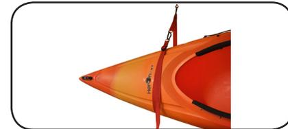
6. Holding the other end of the boat, lock the carabiner to create the opposite support loop. Adjust the boat to confirm balance. Lift the boat and pull the free ends to adjust the height. Never pull the free ends down under the full weight of the boat.
