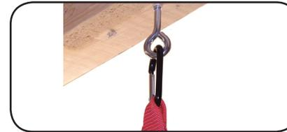
3. Attach the top carabiners with sling assemblies to mounting bolts. Check to confirm that the location of the bolts are high enough off the floor to accommodate the boats. We recommend that you test the strength of each mounting bolt by firmly pulling down on the Straps before continuing with the installation.
