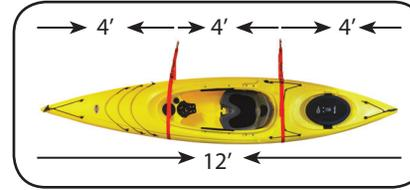
1. To determine the length required between the two ceiling mounting bolts, measure the length of the longest boat to be stored and divide by 3.
