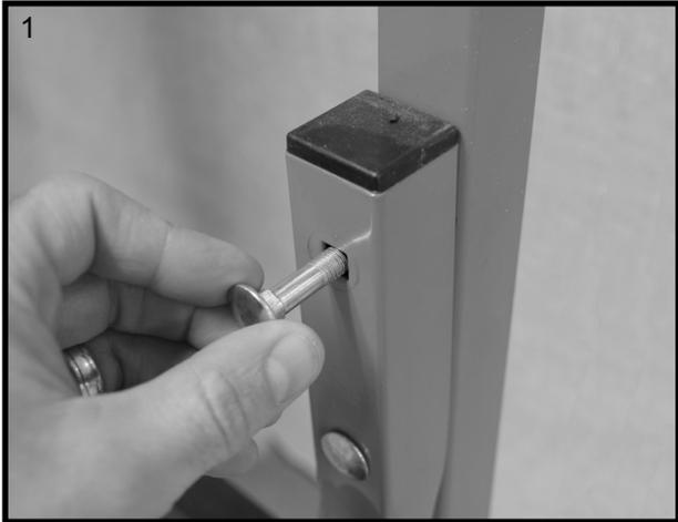
Align the mounting holes in SUP-Style Holder with mounting holes in the uprights of the FS Rack frame. Insert bolts. See image 1.
