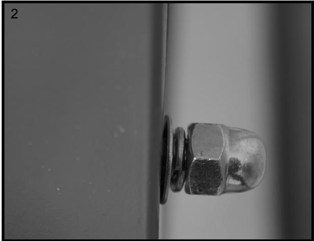
Install larger flat washer first, then the smaller split washer and finally the nut. Use a 1/2 wrench to secure. See image 2.
